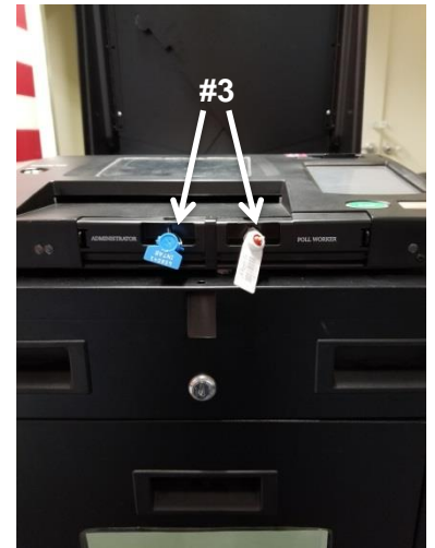
Seal # 3 Compact Flash Door Seals (2)
